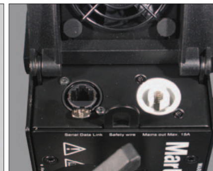
Fig 14: Power and Data output.
